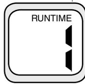
The ICR can be programmed for 8 different run time remote-activated settings (1, 2, 5, 10, 15, 20, 25 and 30 minute increments are available) for the many irrigation functions that may be required. The default setting is 10 minutes.
